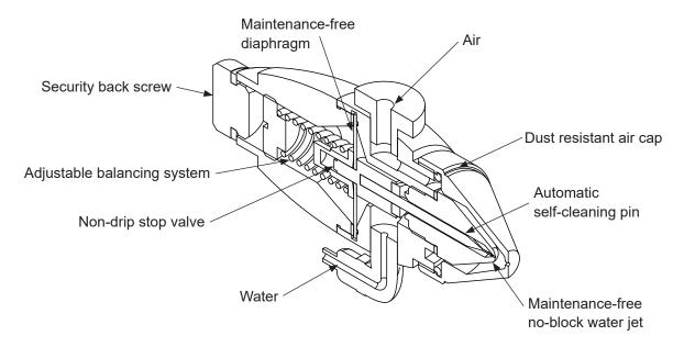
The Jet Spray atomizing nozzles are fabricated in nickel plated brass, incorporating a stainless-steel cleaning pin and diaphragm, with water seal. Air and water under pressure do not mix until they reach the nozzle where they exit at the nozzle tip and atomize to produce a finely atomized spray.
