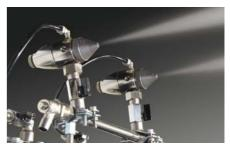
An internal pin prevents blockages, resulting in robust operation in industrial environments. The nozzles come in a variety of outputs and are directionally adjustable, horizontally and vertically.
